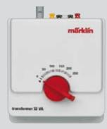
66470 230 Volt Safety Transformer. 32 VA. The track voltage can be adjusted between 4 and 16 volts. The accessory voltage is 16 volts. The transformer has a plastic housing. Dimensions 140 x 120 x 80 cm / 5-1/2" x 4-3/4" x 3-1/8". VDE tested.
