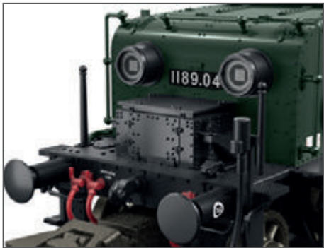
Locomotive ends: striking lamps and the box on the ends typical for this locomotive
